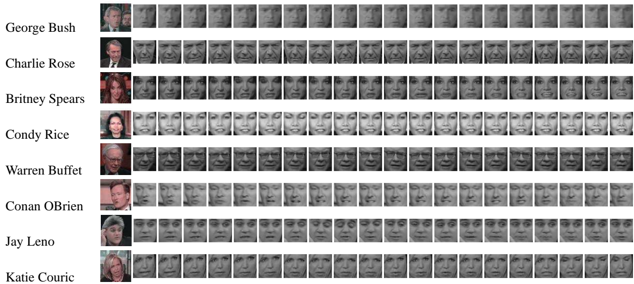
Figure 2: Illustration of face extraction and warping from video frames. Each row shows 20 frames from a chunk. The left most image displays the first frame while the rest of the images display the extracted faces from the subsequent frames warped using thin-plate-spline.
